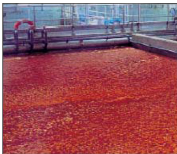
The next step for this sludge produced by a Clari-DAF System is dewatering equipment.
